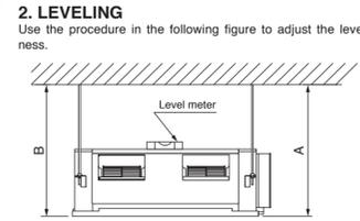
The side A of the unit with the drain port should be slightly lower than the opposite side B of the unit. The height difference between sides A and B should be from 0 to 20 mm.
