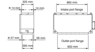
\* Spacing between flange and drain pan.
