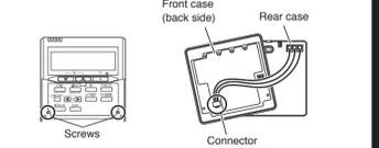
When installing the remote controller, remove the connector from the front case. The wires may break if the connector is not removed and the front case hangs down. When installing the front case, connect the connector to the front case.
