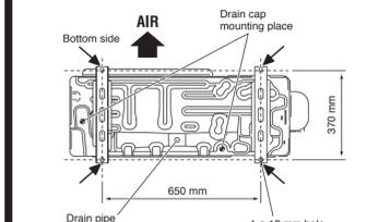
② Fix securely with bolts on a solid block. (Use 4 sets of commercially available M10 bolt, nut and washer.)
