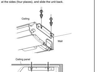
(2) Fasten the indoor unit into place by tightening-up the special "B" bolts and the M10 nuts. Make sure that unit is secure and will not shift back
