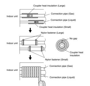
• When using an auxiliary pipe, make sure that the fastener used is insu-
