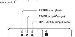
Fhe OPERATION, TIMER and FILTER lamp operate as follows table ac
