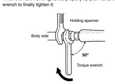
**∴** CAUTION Hold the torque wrench at its grip, keeping it in the right angle with the pipe, in order to tighten the flare nut
