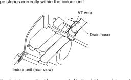
(3) If the drain hose will not be connected to the right rear piping, cut the hole cover at the points indicated in Fig. (a), and attach it to the piping hole as shown in Fig. (b).
